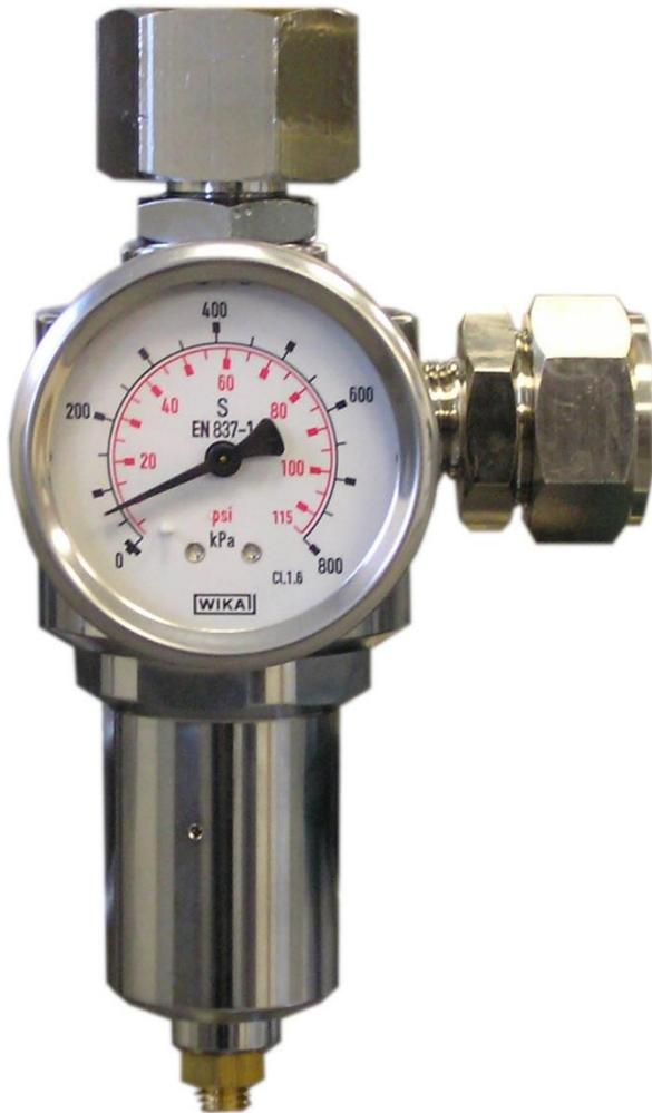
The G8849 regulator is a version of the Gascon Systems MR64 medical oxygen breakdown panel regulator made to suit the G8860 breakdown panel. It is intended for use on the medical facilities bulk oxygen primary gas supply panels.
