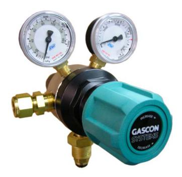
The GS750HF range of regulators offers constant pressure benefits of a two stage regulator. It has a high outlet flow capacity not found in many dual stage regulators. The flow capacity can be up three times that of the C750 regulator range of regulators. The default outlet connection is ½"NPT female that easily allows connection piping up to 1" diameter.
