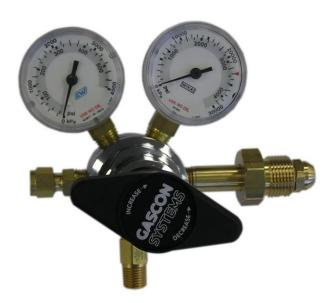
The Gascon Systems extra high outlet pressure regulators are manufactured from brass bar stock and are recommended for use in non-corrosive gas applications. They are ideally suited for industrial work, pneumatic loading of test apparatus, static testing of pressure components, pressurising high pressure systems or high pressure decanting.
